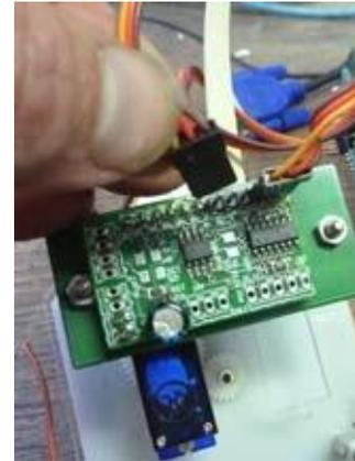
Connect the suction gauge servo to the servo module, left servo connector. **CAUTION TO MEANING**
