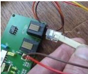
Connect a first bus cable to the master board
