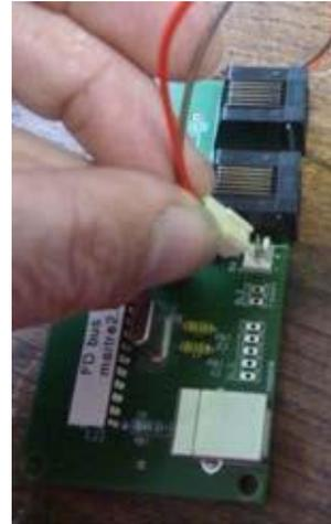
Connect the 5v power supply to the master card
