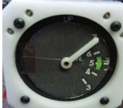
Position cursor 6 to place the needle on marker 6, cursor 7 must be correctly positioned.
