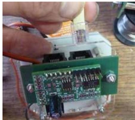
Connect the other side of the cable to the servo module
