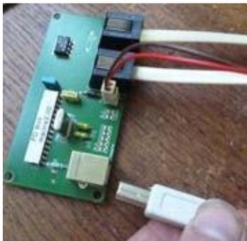
Connect the USB cable to the master card and PC
