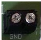
The card has 2 terminal blocks of 2 screw connectors each. That's 4 connectors in total for the common. For the distribution of the GND, you have the choice: a wire that goes from inter to inter, dominoes or terminal blocks.
