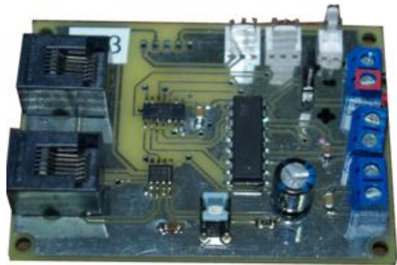
1 motor module FD0024 for motor 800 mA or 1 motor module FD0096 for motor 4,5A
