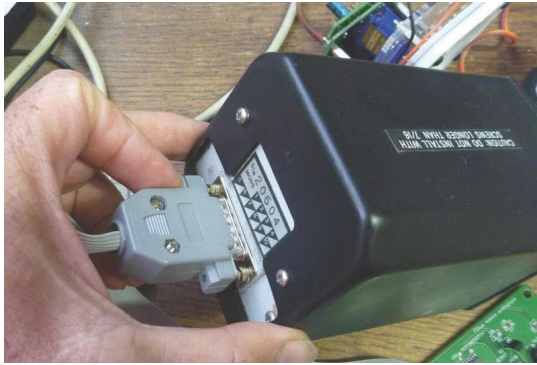
Connect the VOR to the analog card
